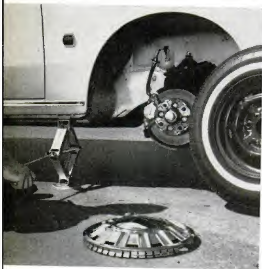
DISC BRAKES up front are standard. Jack fits into special slot, holds car steadier than bumper jacks
